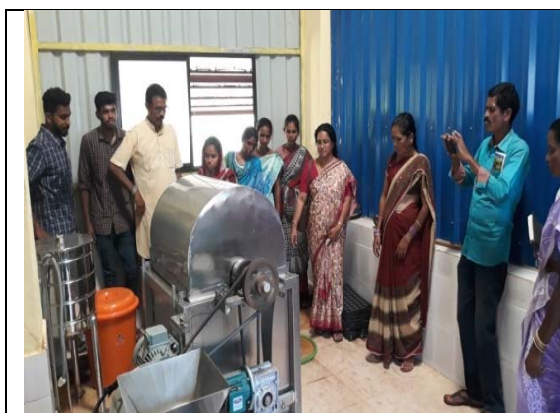
Demonstration of mechanical washer cum peeler for ginger
